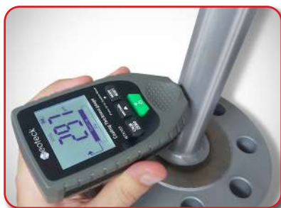
Coating Thickness Check
